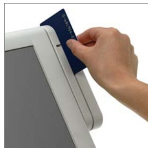
Built-in Magnetic Stripe Reader
